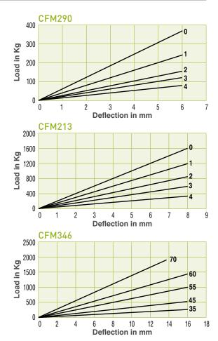
Max compression load in Kg deflection in mm.
