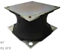
Shear Compression Mountings are manufactured from high quality natural rubber and are designed to allow large amounts of horizontal and lateral movement. They are typically used in the Construction Industry, particularly on Compaction Equipment. The high grade rubber formulation ensures extended service life under continuous high levels of mechanically induced vibration.
