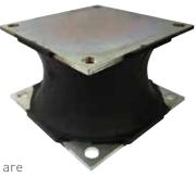
Shear Compression Mountings are manufactured from high quality natural rubber and are designed to allow large amounts of horizontal and lateral movement. They are typically used in the Construction Industry, particularly on Compaction Equipment. The high grade rubber formulation ensures extended service life under continuous high levels of mechanically induced vibration.
