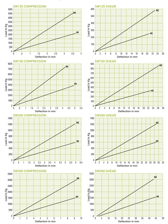
Max compression load in Kg deflection in mm.
