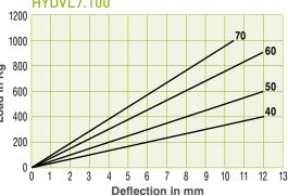
Max compression load in Kg deflection in mm.
