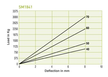
Maximum Loads should be derated for marine propulsion engines. Height adjusters available see page 36
