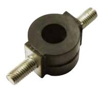
High performance mountings for lightweight equipment. They are designed to give high levels of deflection under light loads, providing a low natural frequency and high levels of vibration isolation – both Active & Passive. They can be used in either compression, shear or a combination.
