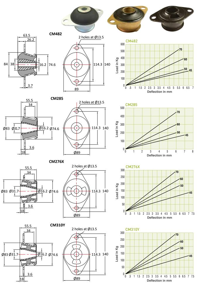
Max compression load in Kg deflection in mm.
